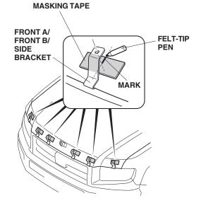
the center of each bracket. Remove all of the brackets from the hood.
