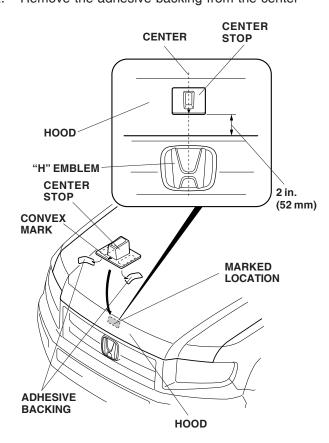
stop, and attach it to the hood at the marked location with the convex mark facing down.
