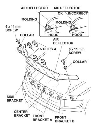
side brackets, and install the two 6 x 11 mm screws and two collars. Tighten the screws securely.
